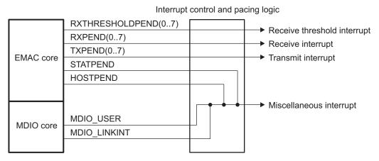
Figure 11. EMAC Control Module Interrupt Logic Diagram
